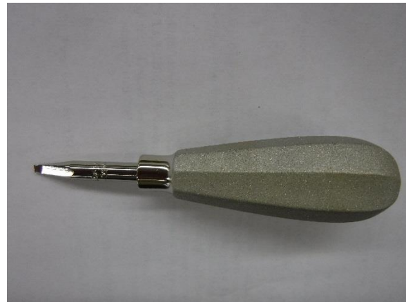
Instrument #1 after 250 dry heat cycles
