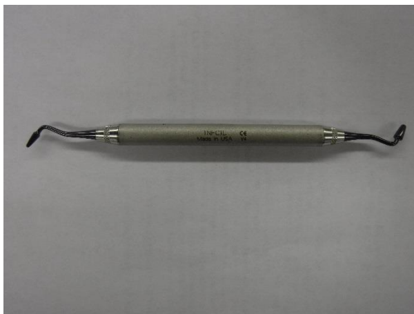
Instrument #2 after 250 test cycles
