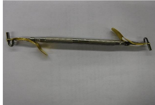
Instrument #4 after 250 test cycles
